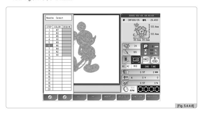
**5** Use the direction buttons and move the cursor to "4" under #7 needle bar. As in <Fig. 5.4.4-9>, the cursor will move to the "4" position.
