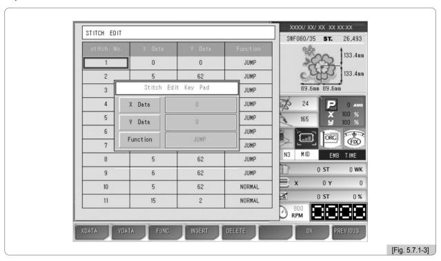
Press F3 FUNC, and as in <Fig. 5.7.1-4>, the menu for setting function codes is enabled.
