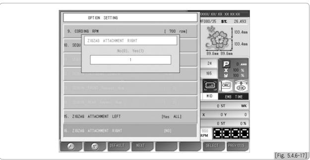
③ In case of setting up of the zigzag on the left side press the number 1 on the number keypad(ex.) at the <Figure 5.4.6-16>, the setting up of the zigzag on the right side is to press number 1 on the number keypad(ex.) at the <Figure 5.4.6-17>.
