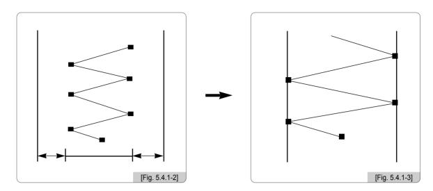
This function determines the satin stitch length in the X-axis direction. The value can be increased by the unit of 0.1[inc].
