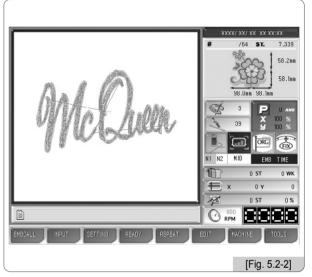
If there are no designs called as in <Fig. 5.2-1>, several function buttons cannot be used. The buttons whose letters are pale cannot be used until the designs are called later.
