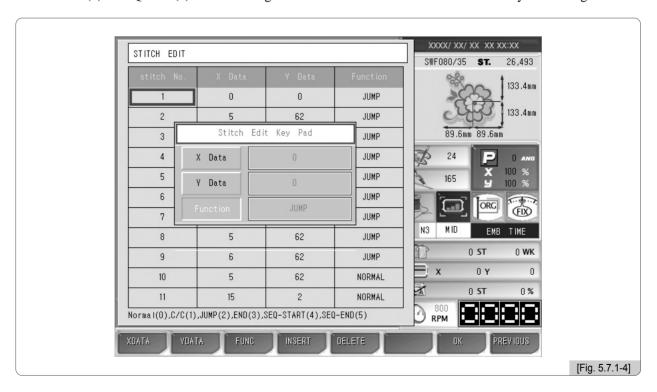
Set the [4] INSERT key when adding the needle data and set the [5] DELETE key when deleting the needle data.
