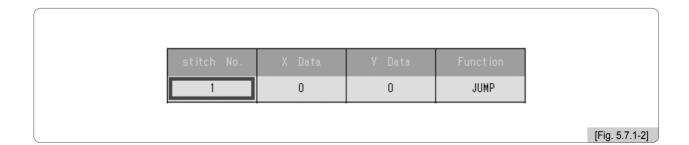
Press  $\boxed{\text{F1}} \times \text{DATA}$ ,  $\boxed{\text{F2}} \times \text{DATA}$ . And as in <Fig. 5.7.1-3>, it is possible to correct X, Y data. Use the number keys to enter values.
