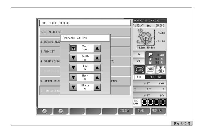
When the cursor is located at  $\ lacktriangledown$ , press  $\ lacktriangledown$  for date and time.
