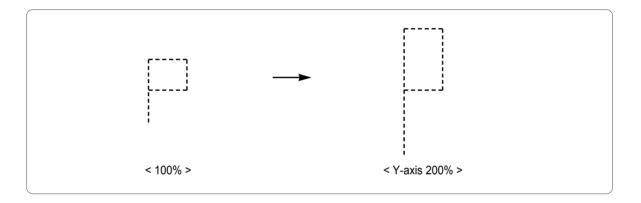
The default is 100%, and the value can be adjusted from 50% to 200% by the unit of 1% .
