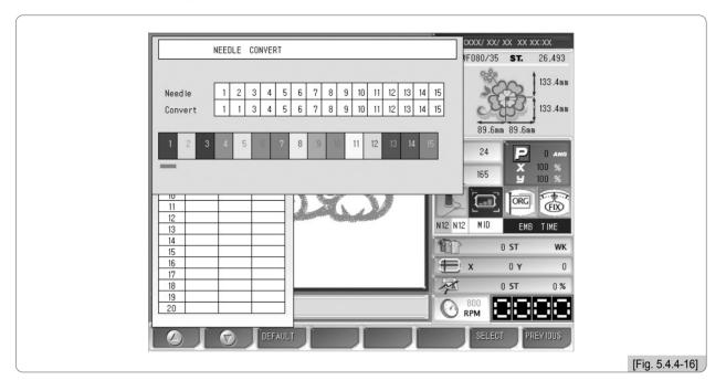
Move the needle bar you want with the [1] keys and select, then the screen to choose colors like <Figure 5.4.4-17> is displayed. Go to the color you want by using the [1] , [2] , [2] , [2] , keys and press the [7] SELECT key, then lower part of color identification chanes into selected color(upper part of color identification is the color before setting up). The selected color is saved when pressing the [8] ANTERIOR key.
