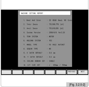
Use  $\boxed{1}$   $\bigcirc$  to move to a desired item and press  $\boxed{7}$  SELECT . Then the screen like 'Fig. 3.2.1 Embroidery Machine Specifications Setting' appears where the setting of each item is possible. When the setting is completed for all items, press  $\boxed{7}$  NEXT . <Fig. 3.2.0-2> appears to check the set specifications.
