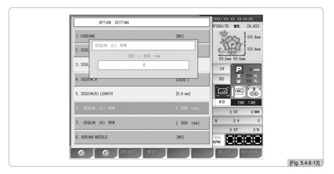
① Enter a desired figure within the setting range of 300rpm~800rpm using the keypad.
