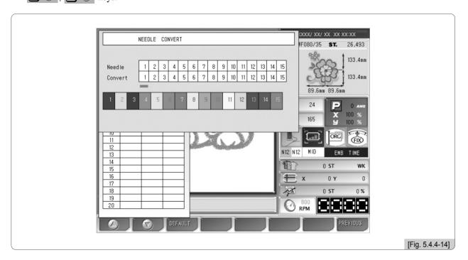
Fress the number 1 on the number keypad after moving to No.2 needle bar. Like <Figure 5.4.4-15>, the needle bar is moved from No.2 position to No.1 position.
